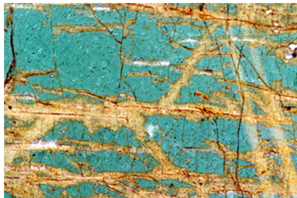
Fig. 4. The oxidation of green hagendorfite to yellow alluaudite. Kibingo pegmatite, Rwanda. The length of the picture represents 3 mm.
