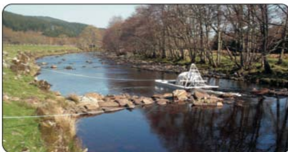
Rotary screw trap in operation on a tributary of the River Conon
