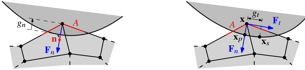
(a) Normal contact interaction. The normal contact force \mathbf{F}_n is proportional to the small normal overlap g_n .
