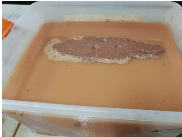
Unstabilized CEBs (0 % CCR)
