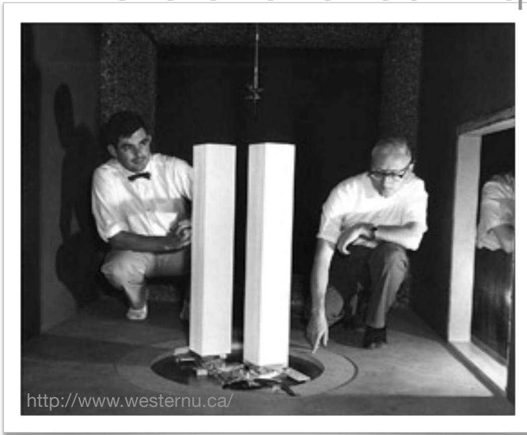
1964: Wind Tunnel Testing World Trade Center (Drs. J.E.Cermak and A.G. Davenport in the Colorado State University boundary layer wind tunnel)
