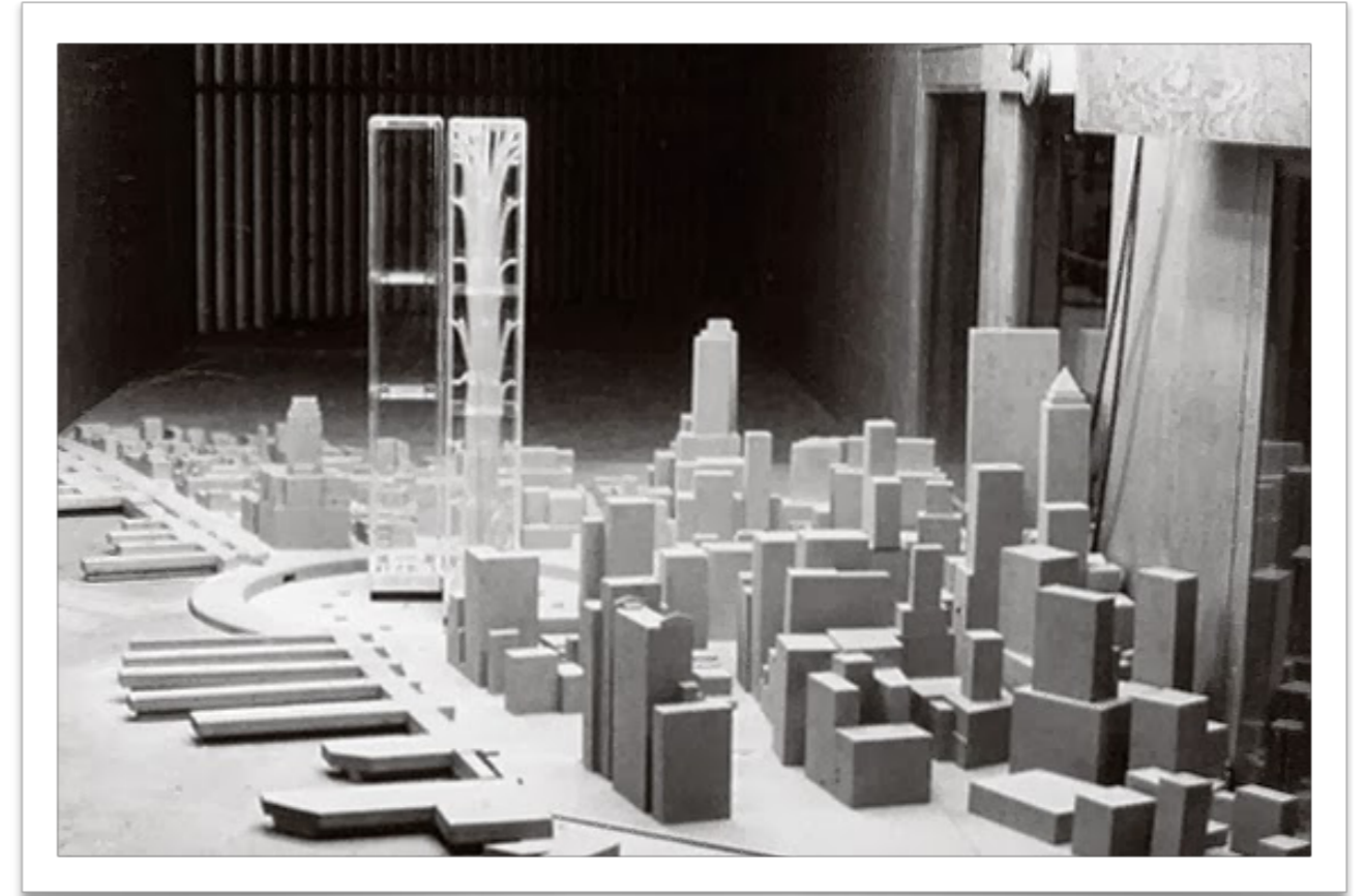
1964: Wind Tunnel Testing World Trade Center (Drs. J.E.Cermak and A.G. Davenport in the Colorado State University boundary layer wind tunnel)
