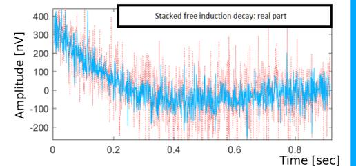
Fig. 1: Example of a SNMR Free Induction decay signal
