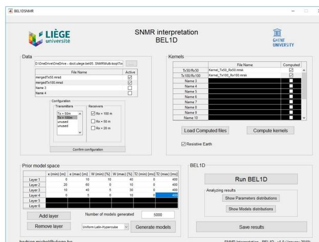
Fig. 4: Graphical user interface for the interpretation of SNMR data through BEL1D (available on GitHub)
