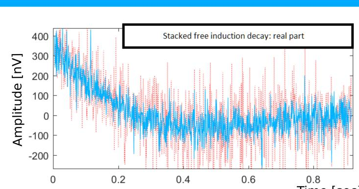
Time [sec] Fig. 1: Example of a SNMR Free Induction decay signal
