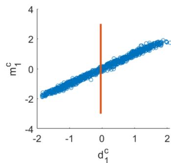
Fig. 2: Extract of the statistical relationship obtained through BEL1D
