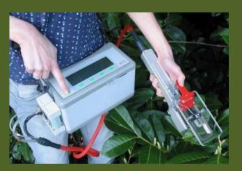
Infra-red gas analyser photosynthetic rate (A)
