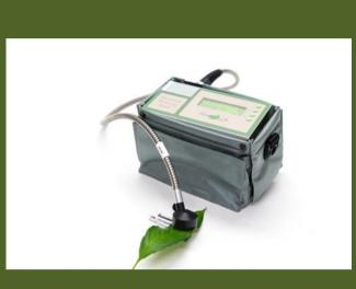
Fluorimeter quantum efficiency of photosystem II (Fv/Fm)
