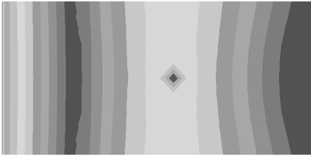
**Figure 4:** clamped (on the right side) plate with a very thin square zone, (mode 3)
