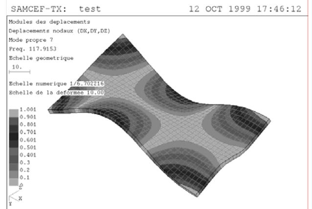
**Figure 2**: FE results (Mode 7 at 117.9 Hz)
