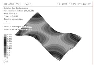
Figure 2: FE results (Mode 7 at 117.9 Hz)
