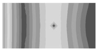
Figure 4:clamped (on the right side) plate with a very thin square zone, (mode 3)
