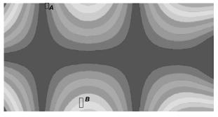
*Figure 1 : Simulated optical measurements (Mode n° 7 at 116.25Hz). (Fixations are on the right side.)*
