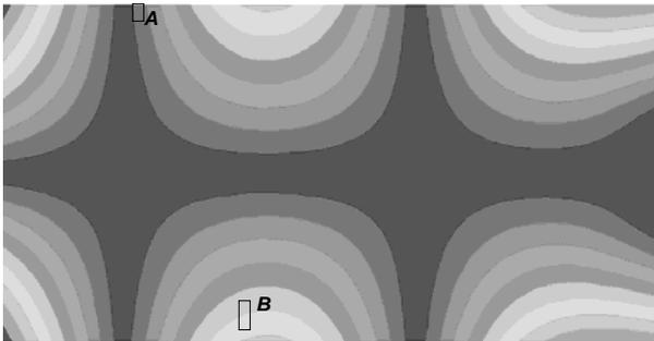
**Figure 1** : Simulated optical measurements (Mode n° 7 at 116.25Hz). (Fixations are on the right side.)
