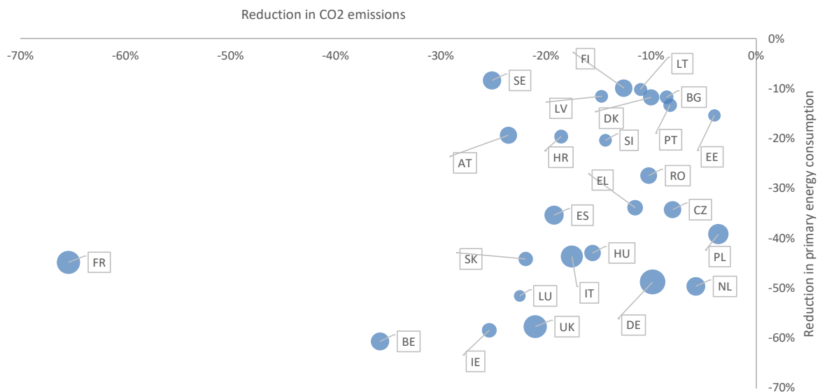
Figure 9: Comparison of current case and a full electrification scenario. Bubble size are proportional to the useful energy demand of each country
