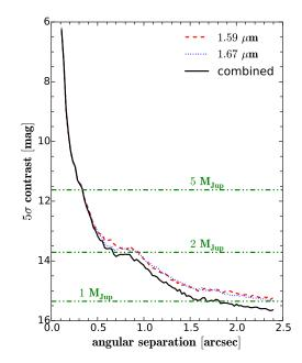
**Fig. 8.** Azimuthally averaged detection limits for the SPHERE ADI observation reduced with the TLOCI algorithm. We give the  $5\sigma$  detection limit in magnitudes. Assuming an age of the system of 2.5 Myr and a distance of 158 pc, we calculated mass detection limits using the BT-SETTL model isochrones (green dash-dotted lines).
