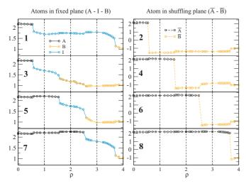
FIG. 5. (Color online) Evolution of the local magnetic moment for the eight atoms of the supercell as a function of the reaction coordinate  $\rho$ . The black, orange, and blue colors approximately depict the bcc, hcp, and mixed bcc/hcp values for the magnetic moment. The atom numbering is related to Fig. 4. Atoms 1, 3, 5, 7 belong to the A layers, and atoms 2, 4, 6, 8 are successively moving from an  $\bar{\text{A}}$ -type layer to a  $\bar{\text{B}}$ -type one.
