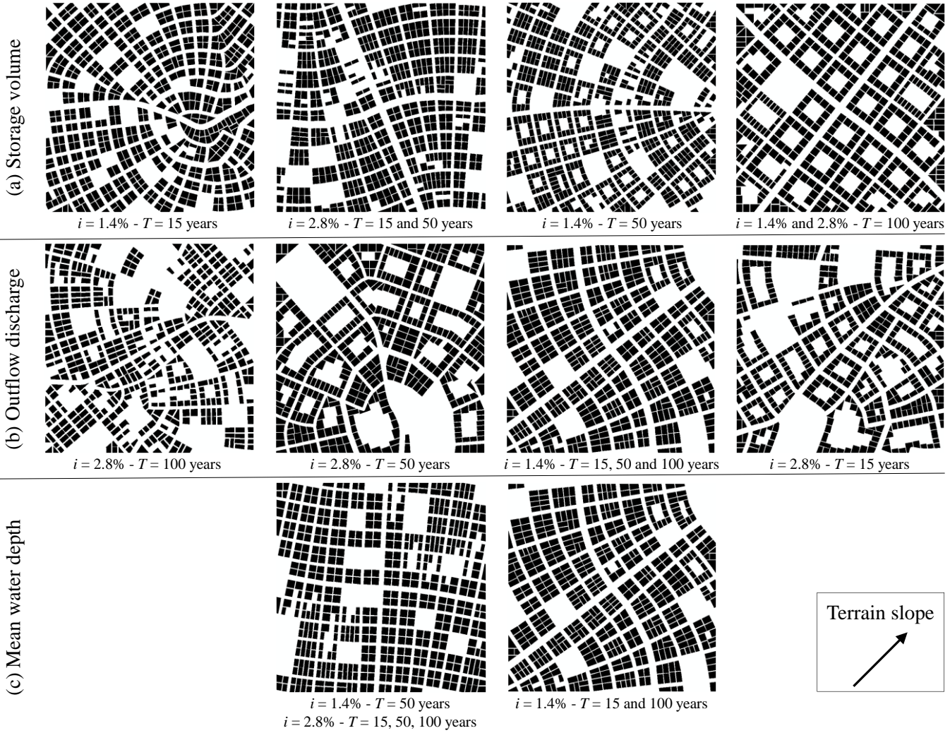
417 Figure 8: Building footprints in the urban forms leading to the minimum peak values of the stor- 418 age volume (a) and maximum peak values of the outflow discharge (b) and mean water depth (c) 419 for the different terrain slopes i and return periods T .
