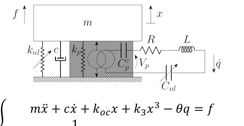
The piezoelectric patches are shunted by circuits with nonlinear capacitors having different functional forms. Clearly, the absorber obeying a principle of similarity [4] is the one which exhibits the best performance.
