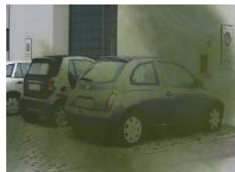
Typical failure: ghosts
