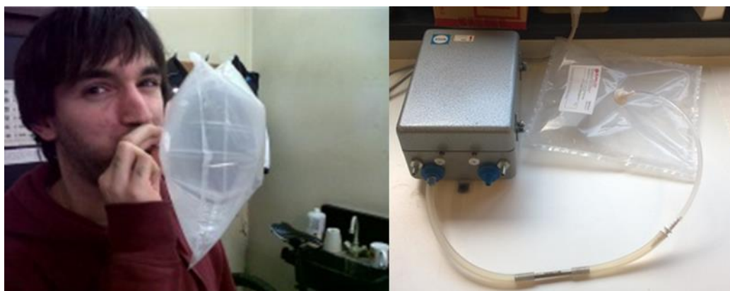
Figure 29: Representation of the exhaled breath sampling with on the left the collection of breath in Tedlar® bag and on the right the transfer on TD tube via a pump
