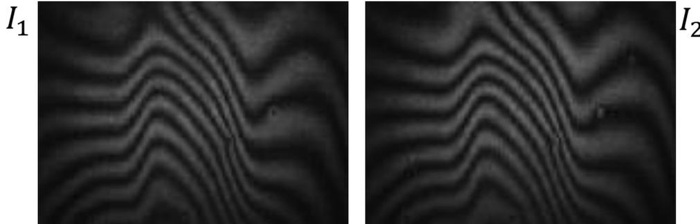
$$\phi = \arctan\left(\frac{I_4 - I_2}{I_1 - I_3}\right)$$
