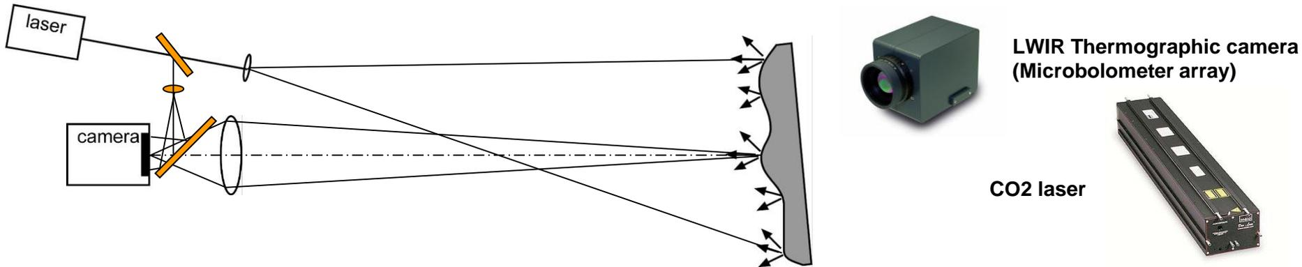
$$Sp_{LWIR}(x, y) = I_{thermal}(x, y) + I_o(x, y) + I_r(x, y) + 2\sqrt{I_o I_r} \cos(\psi(x, y))$$
