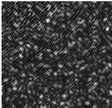
$$Sp(x, y) = I_O(x, y) + I_R(x, y) + 2\sqrt{I_O I_R} \cos(\psi(x, y))$$
