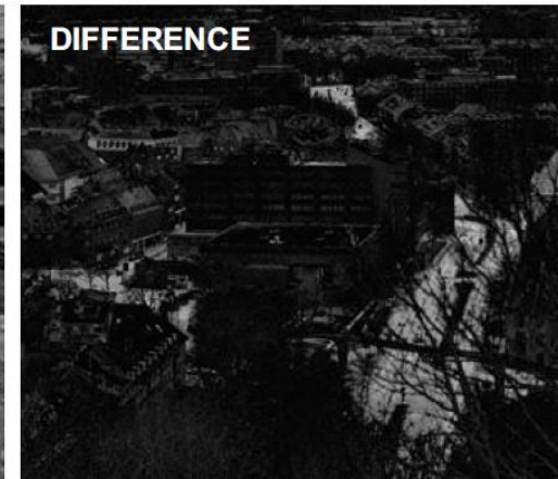
Streets exhibit higher intensity in the MWIR, and appear clearly when both images are subtracted
