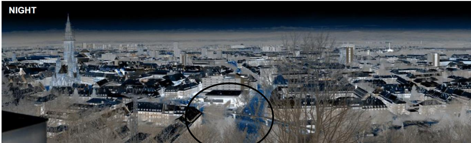
Dual-band IR images of the city of Freiburg (Germany). Contrast and details are enhanced by overlaying both MWIR and LWIR images with complementary colors.
