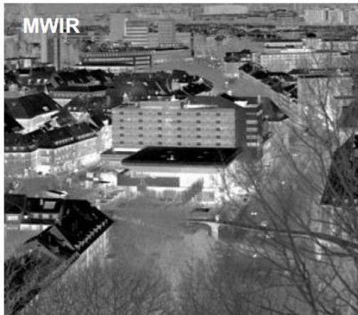
Streets exhibit higher intensity in the MWIR, and appear clearly when both images are subtracted
