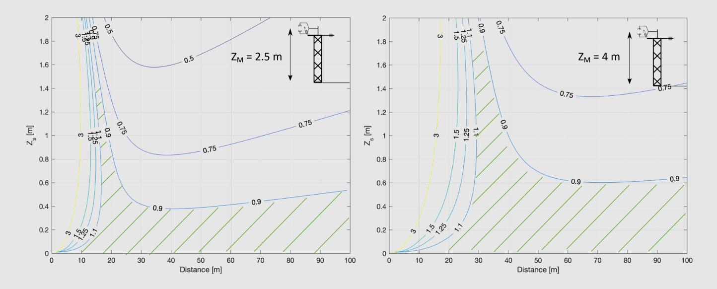
It exists a domain depending on the source height and the distance from the mast for which neglecting the source height induce a small error on the footprint (<10%). This domain is affected by the mast height.
