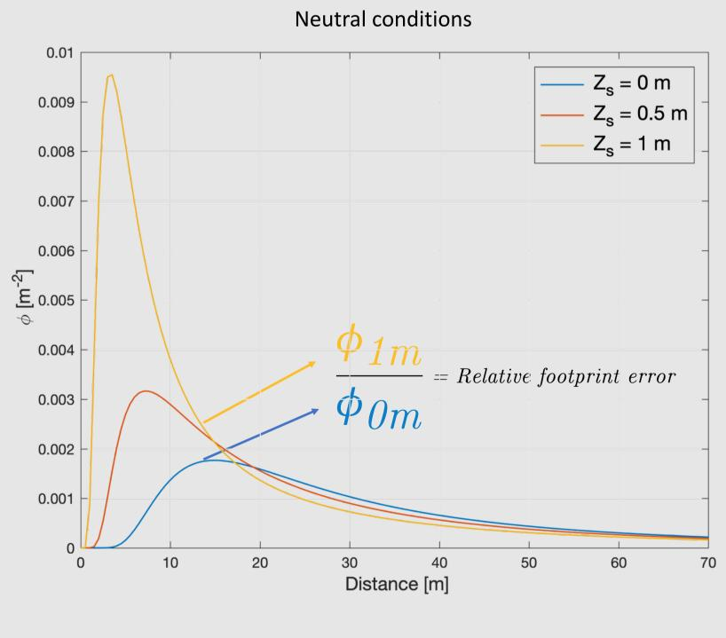
When the source height increases, the footprint peak shifts toward the mast and the peak magnitude increases. This behavior is observed for each atmospheric conditions.
