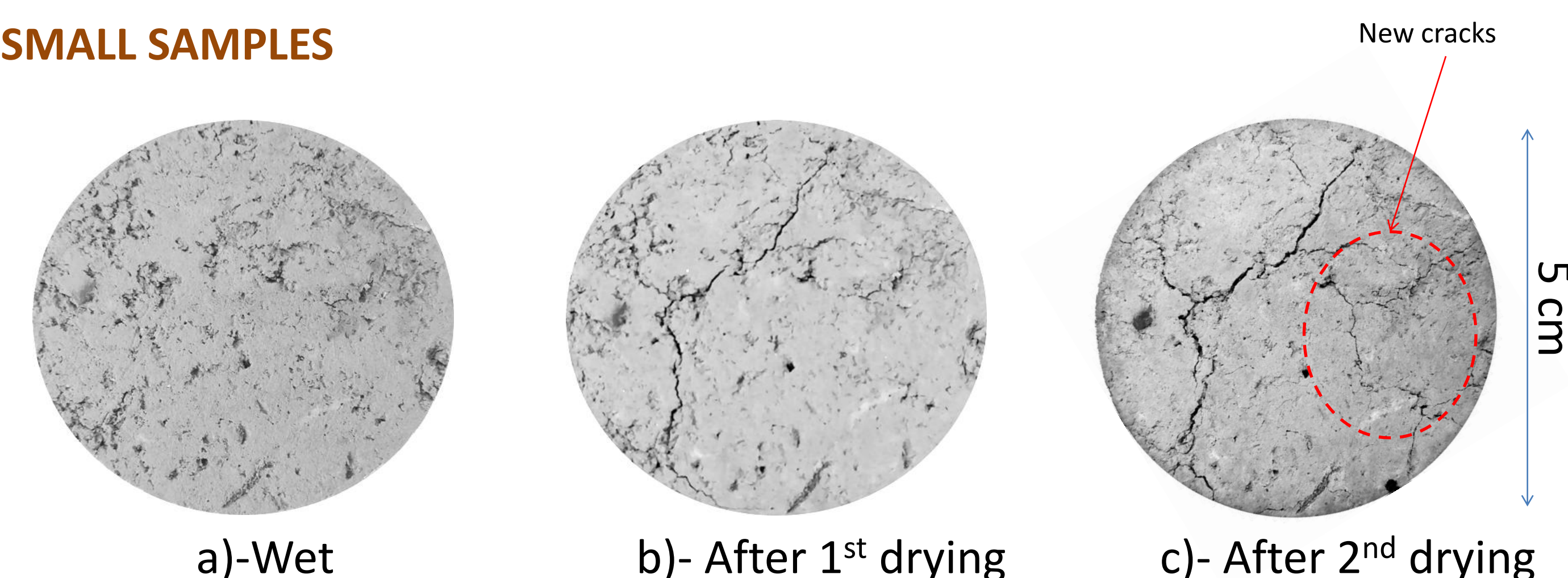
Figure 3: Cracks formation from wet (a), to first (b) and second (c) dryings of small samples
