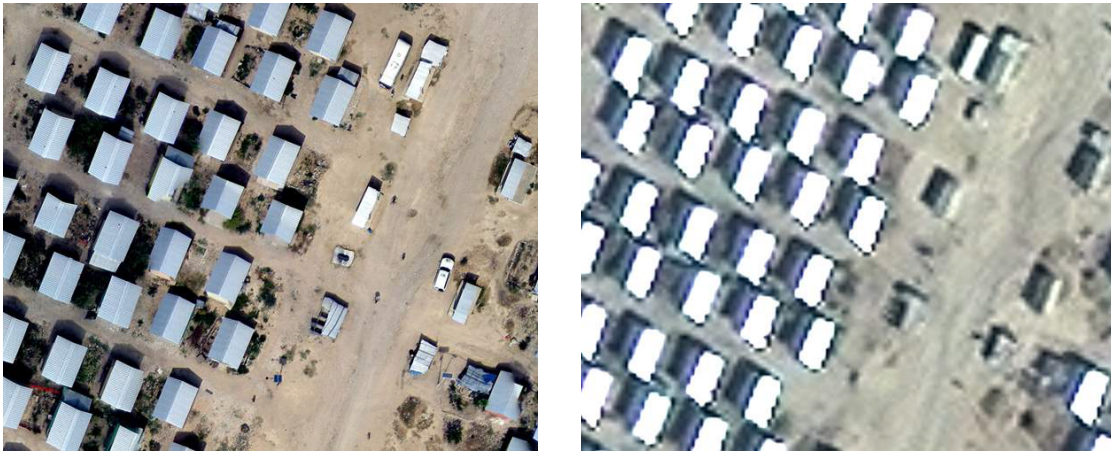
FIGURE 1.1: High-resolution drone images (left) and lower-resolution satellite images (right). From [Swiss Foundation for Mine Action, 2016].
