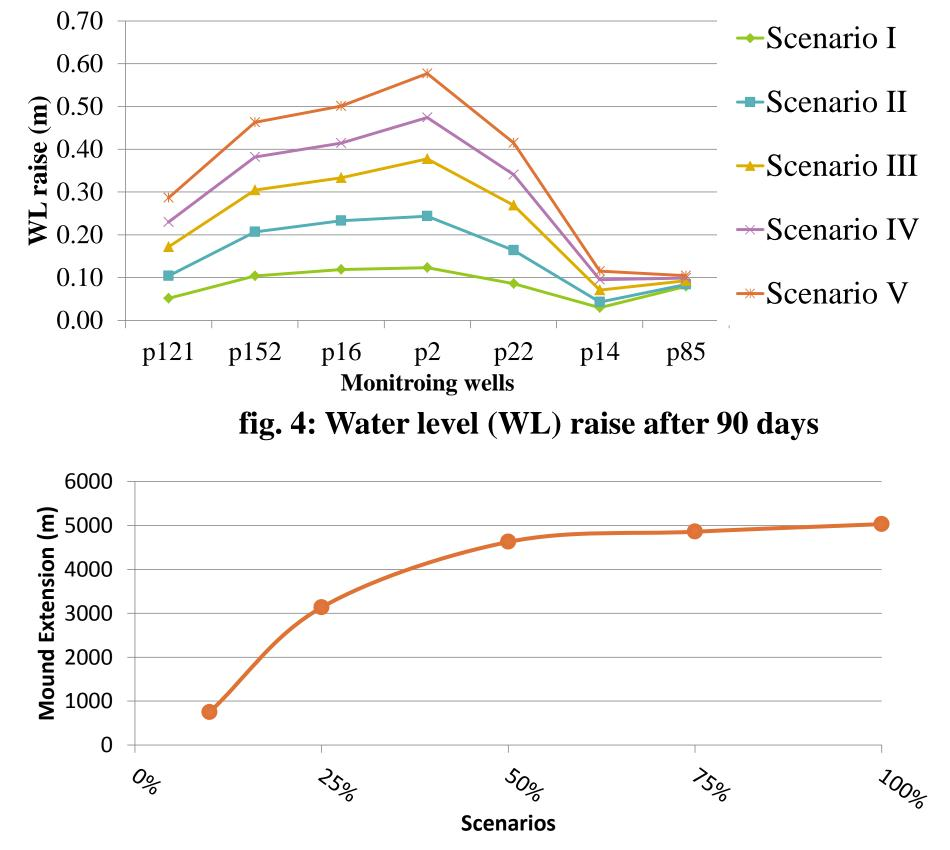
management of surficial and underground water . Hence, a **conceptual groundwater model** of the shallow aquifer is built using the Modflow-2000 under GMS GUI software.
