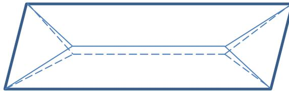
Figure 1: failure mode according to the yield line theory
