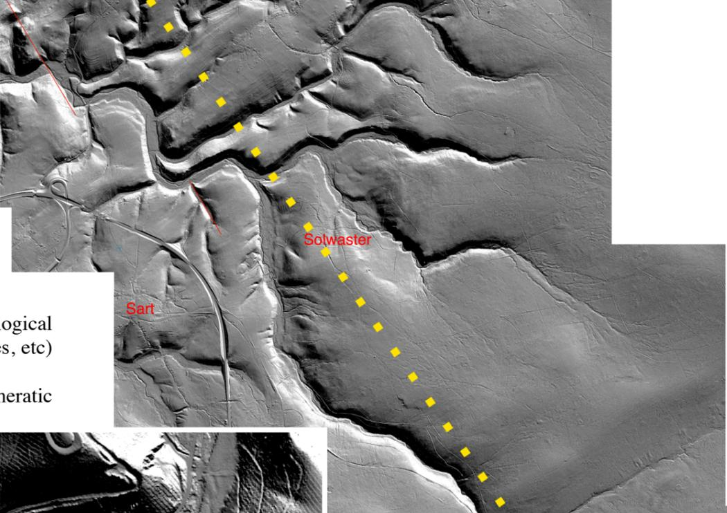
Lidar image (MNT 2013-2014 "Hillshade" from the Public Service of Wallonia internet site "WalOnMap"). Image composition along an active tectonic zone, the Hockay Fault Zone (yellow interrupted line) showing landslides areas (blue zones).
