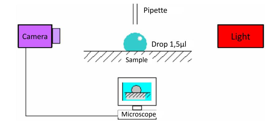
Deposit of the drop (left) and reading of the contact angle (right)
