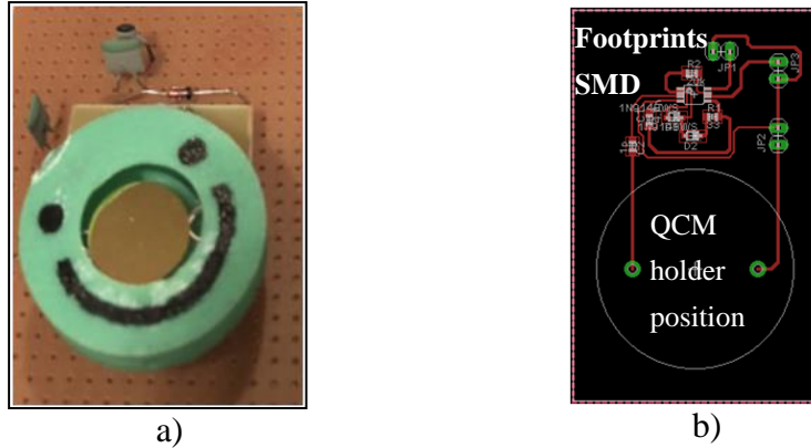
Figure 6. 5: Actual circuit of the high speed peak detector. a) Prototype board. b) Proposed PCB layout design.
