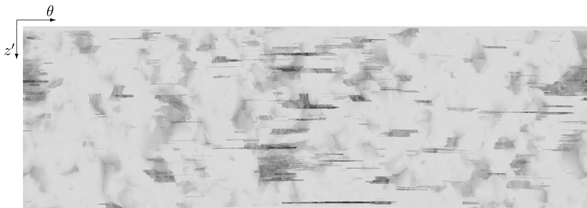
(d) Distance map \mathcal{D}(\mathcal{P}, \mathcal{T}) (since this 2D image is in polar coordinates, the horizontal and vertical axes are respectively the angle around and the distance along the sample's axis (and not the z -axis of the tomography))
