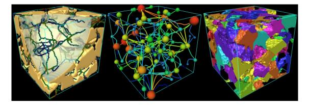
Illustration of a decomposition process: the left image shows a portion of the porous material with the skeleton of the pore space. The centre image is a graph representation of the skeleton, and the right image the result of a region growth using the nodes of the graph.
