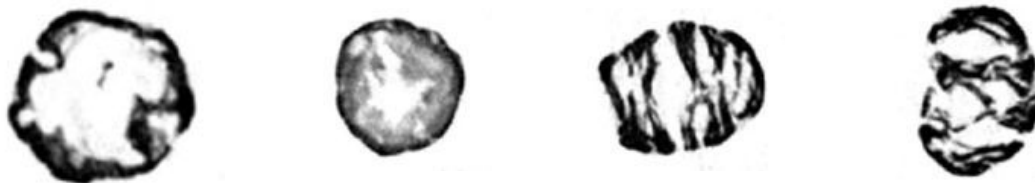
Fig. 4. 2D cross section of dried sludge samples dewatered using different coagulant/flocculant combinations (from left to right) (Pambou, 2016)
