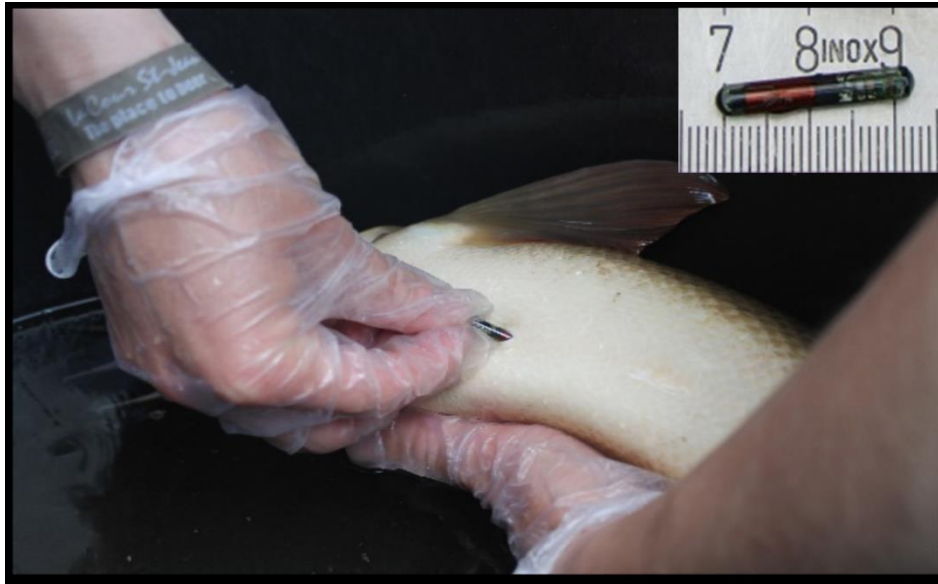
Fig.2 : Transpondeur RFID (Texas Instrument)
