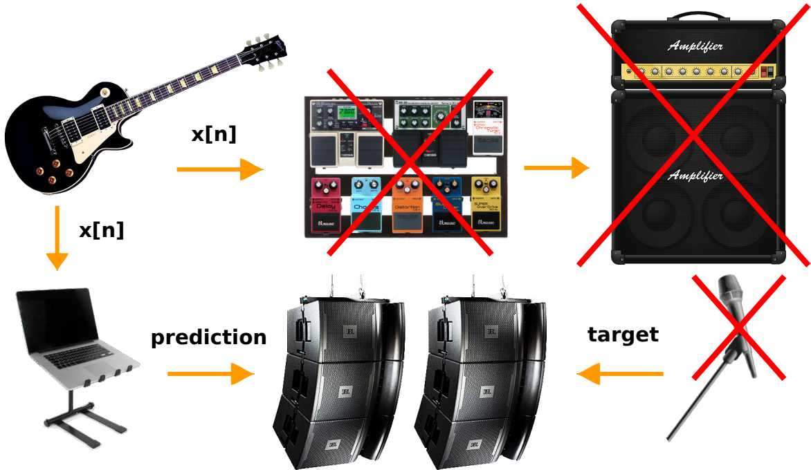
Figure 1.3 Replacement of a typical guitar signal chain by a computer emulation.
