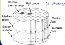
Probing the magnetic field inside the holes
