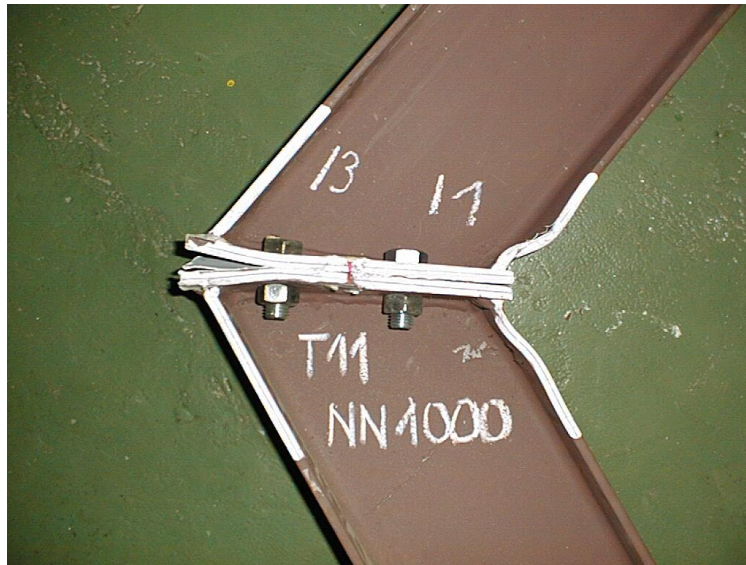
Fig. 12 - Flush end-plate joint NN1000 (Prague) at collapse, yielding of the end-plate in bending (EPB) and of the beam flange and web in compression (BFC) [9]
