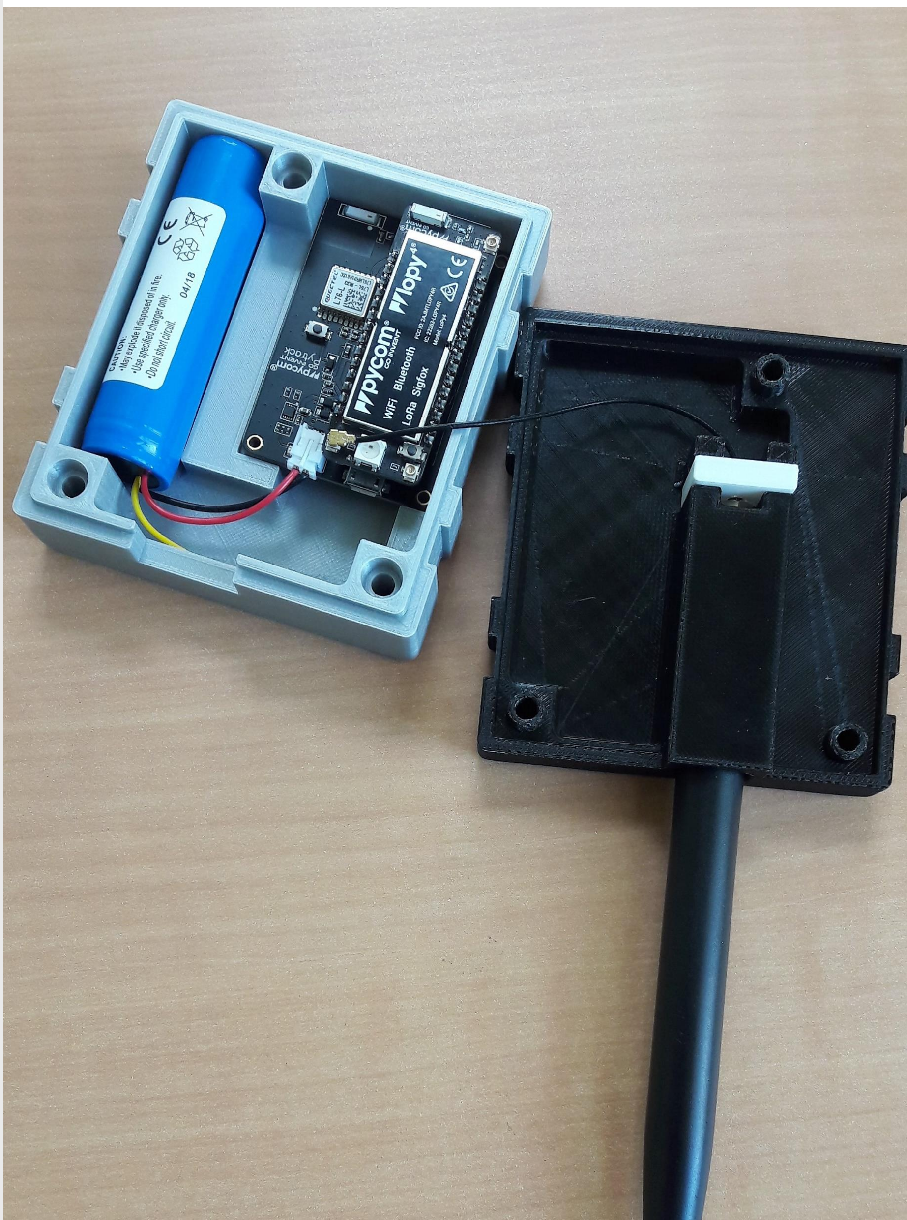
Figure 4: mobile LoRaWAN device with its custom packaging.
