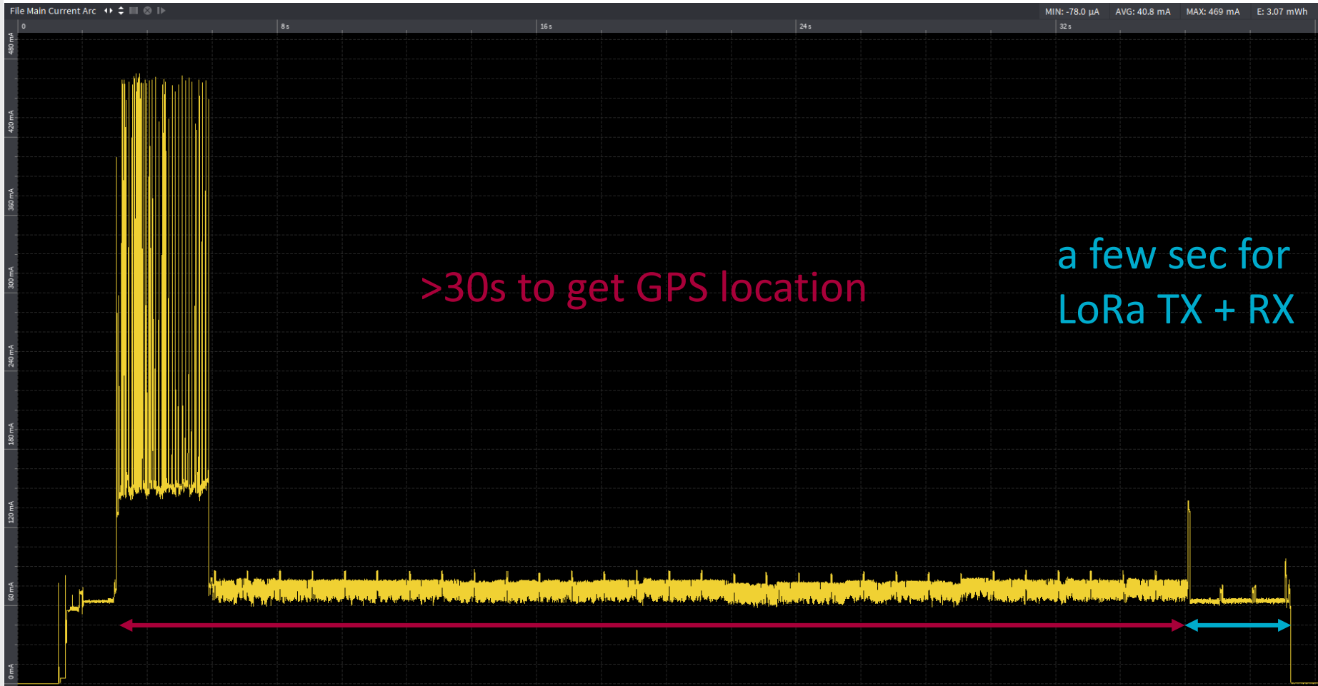
Figure 3: current consumption profile of a GPS locator tag
