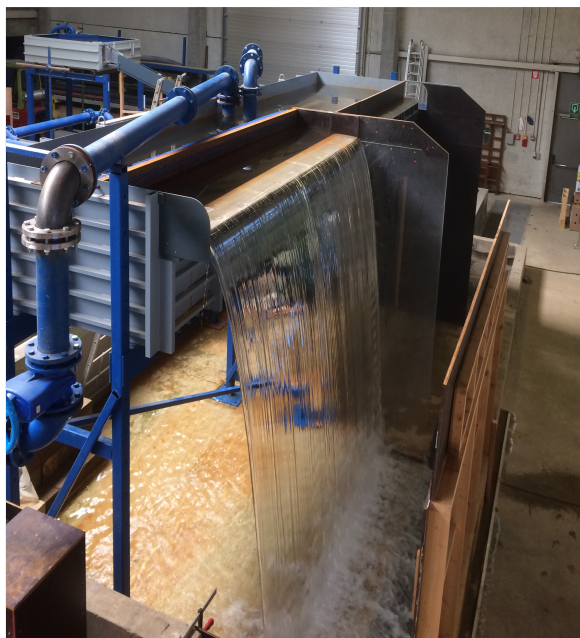
Figure II.2: View of the prototype scale model – Model 1 with flow over the unconfined weir
