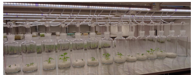
Fig. 1 Epoxiconazole dose-response experimental set-up with two 93 oilseed rape plantlets (at the 21-day-old stage) with home-made cuvette 94 system using perlite substrate
