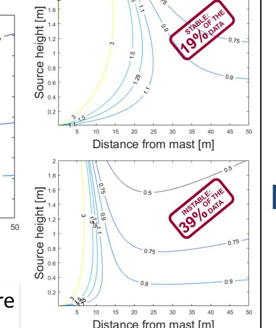
For distances larger than 10 to 20 m (mast height of 2.6 m) emissions are underestimated by up to 25% if the source height is not considered.
