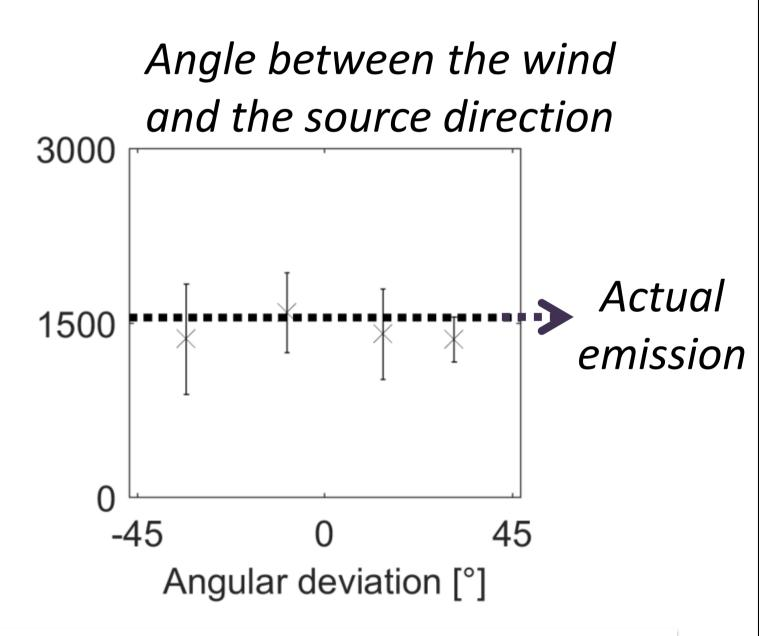
Estimated methane emissions were robust, no matter the atmospheric stability, the distance from the mast or wind direction relatively to the source
