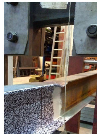
Fig. 6. Force-displacement of the control point (1C) and local deformation of the beam at the end of tests ITB06 M1 H3000.
