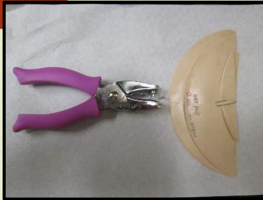
Step1: Punch the handsheet to obtain 3 mm (diameter) paper discs
