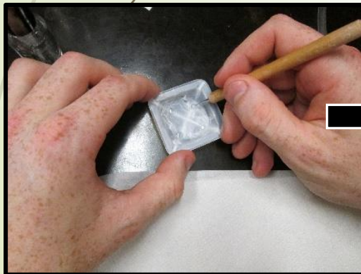
Step 4: Put a small dot of transparent nail polish into the bottom of a well.
