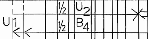
C<sub>p</sub>  $C_{pm} = \frac{1}{2} B_{4m} + U_{1m} - \frac{1}{2} U_{2M} = 2$  (part du brut)  $U_2 = 120 \begin{smallmatrix} +0,4 \\ 0 \end{smallmatrix}$
