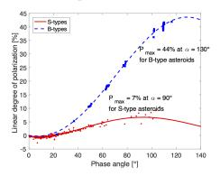
Typical phase-polarization curves for NEAs of S and B type (M. Devogèle, 2018)
