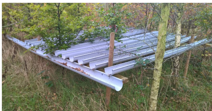
Figure 13. Rainout shelter in Zedelgem. Twenty-four similar drought subplots were installed with a plot size of 3m x 3m and heights in the upper and lower site of 0.95 m and 0.75m, respectively.
