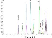
Fig. 4. Spectra of 1  $\delta$ -tocopherol 2  $\beta$ - $\gamma$  tocopherol 3  $\alpha$ -tocopherol 4 brassicasterol, 5 campesterol,  ${\bf 6}$  stigmasterol,  ${\bf 7}$   $\beta\text{-sitosterol}$  using a conventional C18 column. Run time of 6.5 minutes
