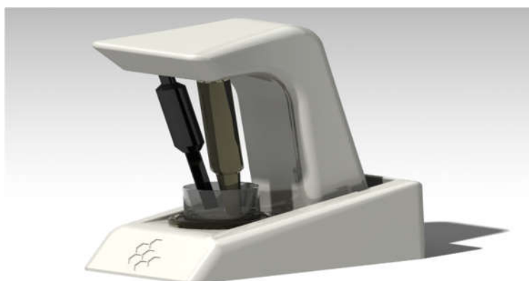
Figure 1. Photography of the PAOT-Liquid® Technology device showing both reference and working microelectrodes immersed in the reaction medium containing free radical mediator M^* and antioxidants or wines samples.
