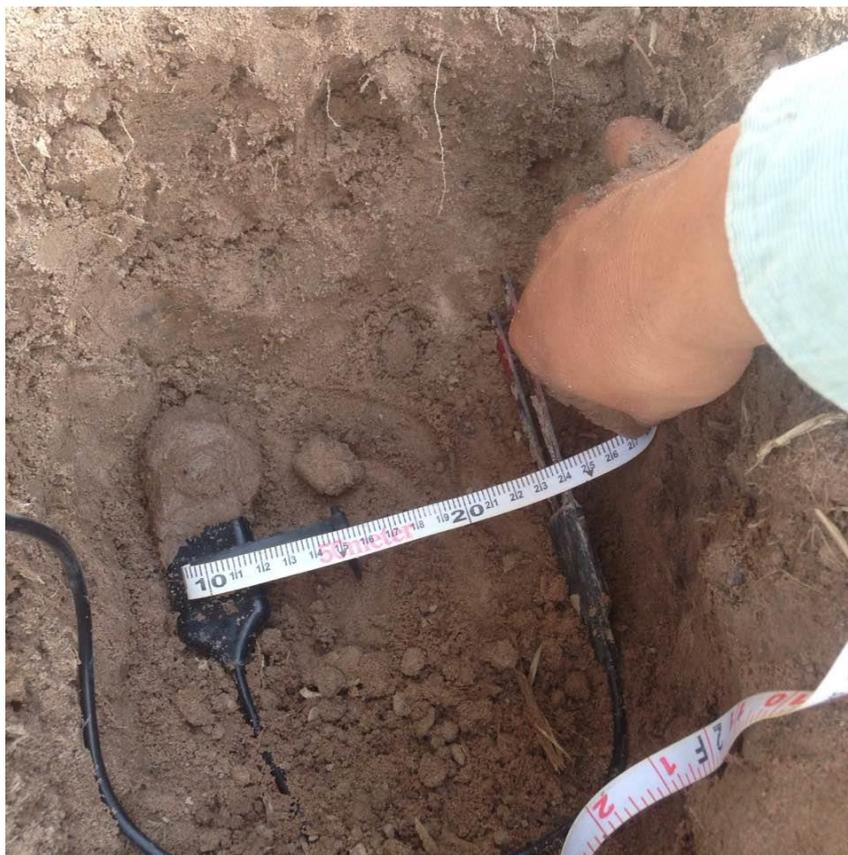
**Figure 3.3-5** In-situ soil water retention curve measurement with a combination of 10HS and MPS-2 sensors. Installation of sensors (the picture was taken before inserting the sensors into the soil) at 10 and 20 cm depths.
