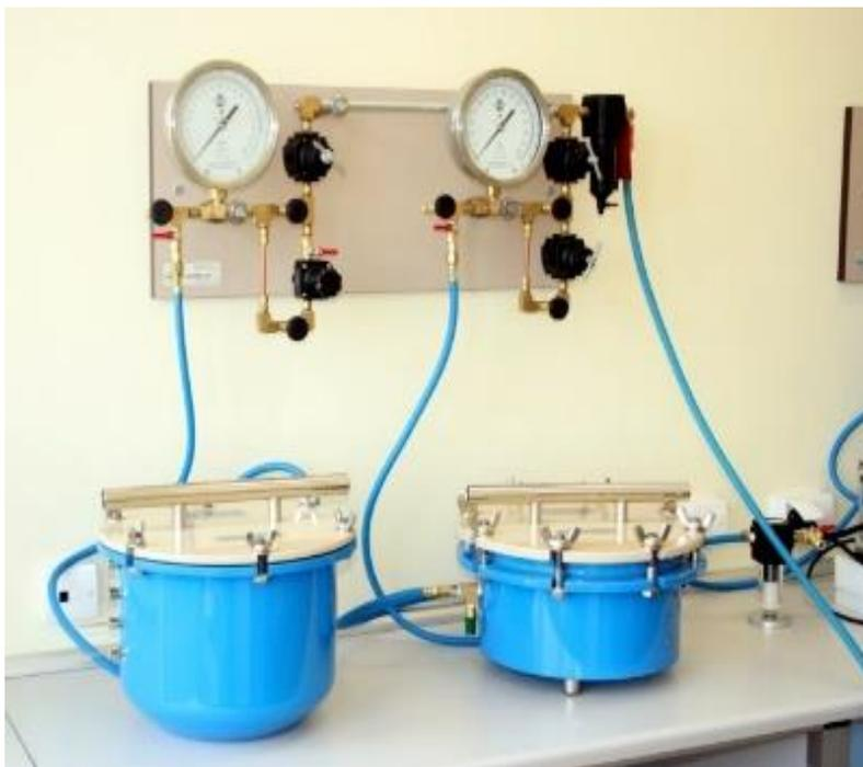
**Figure 3.3-4** pF cure measurement with ceramic pressure plate.
