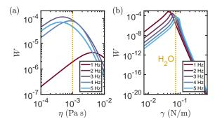
**Fig. 5.** (a) Swimming efficiency W of the collinear magnetocapillary swimmer as a function of viscosity, for various values of the excitation frequency f. (b) Swimming efficiency W of the collinear magnetocapillary swimmer as a function of surface tension, for various values of the excitation frequency f. The contact angle between the spheres and water was kept constant.
