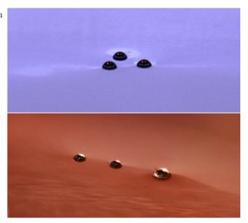
Fig. 3. On top, a triangular magnetocapillary swimmer, composed of three 500  $\mu$ m spheres floating on water submitted to a vertical field  $B_z \approx 3$  mT. On bottom, a collinear swimmer composed of two 400  $\mu$ m and one 500  $\mu$ m sphere. In this case we have a vertical  $B_z \approx 5$  mT and horizontal  $B_x \approx 3$  mT.
