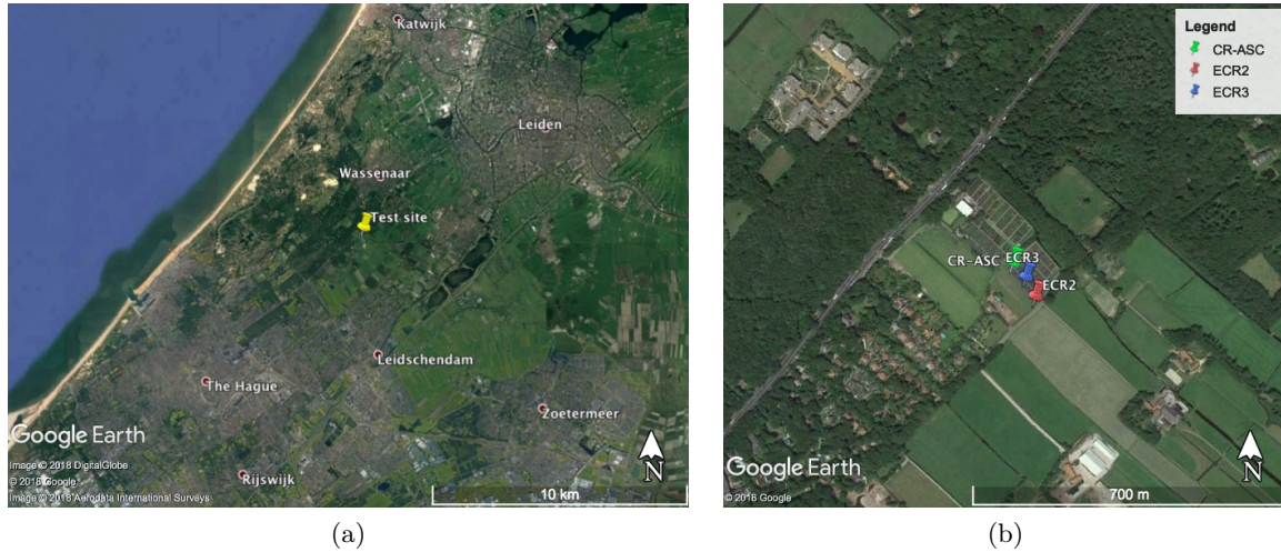
Figure 4.2: Google Earth TM views of the Wassenaar test site. (a) Location of the test site indicated by the yellow pin. (b) Locations of the artificial reflectors. The green, red and blue pins indicate respectively the locations of the ascending corner reflector (CR-ASC), the transponder No. 2 (ECR2) and the transponder No. 3 (ECR3).
