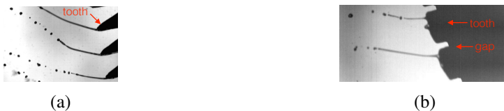
Figure 5.1: Illustration of the formation of jets at the disk border of two CDA atomizes: (a) Case of the Micromax 120 (Micron) (b) Case of the Girojet (Tenoma)
