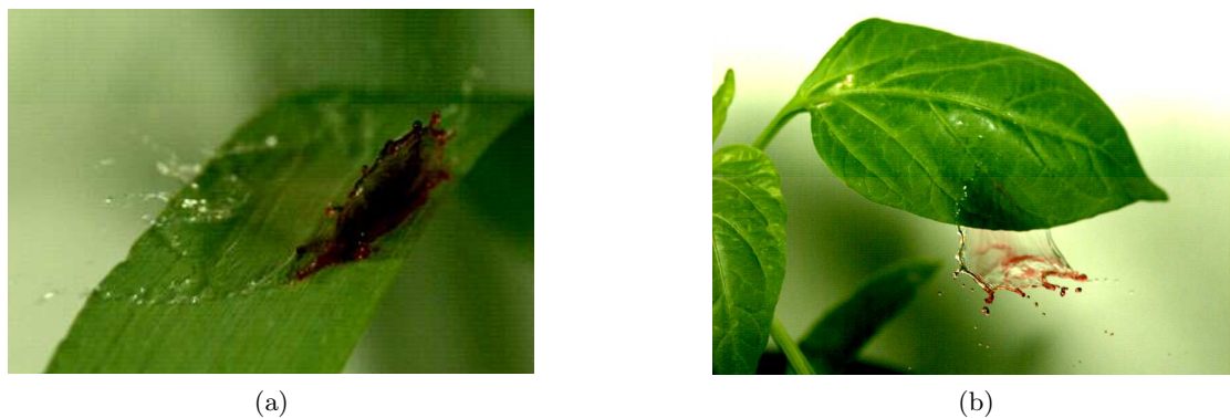
Figure 1.6: (a) Crescent-moon scenario. A clear water drop impacts in the vicinity of a red dyed droplet sitting on a grass leaf. (b) A clear water drop impacts directly on a red dyed water residue sitting on a pepper leaf.
