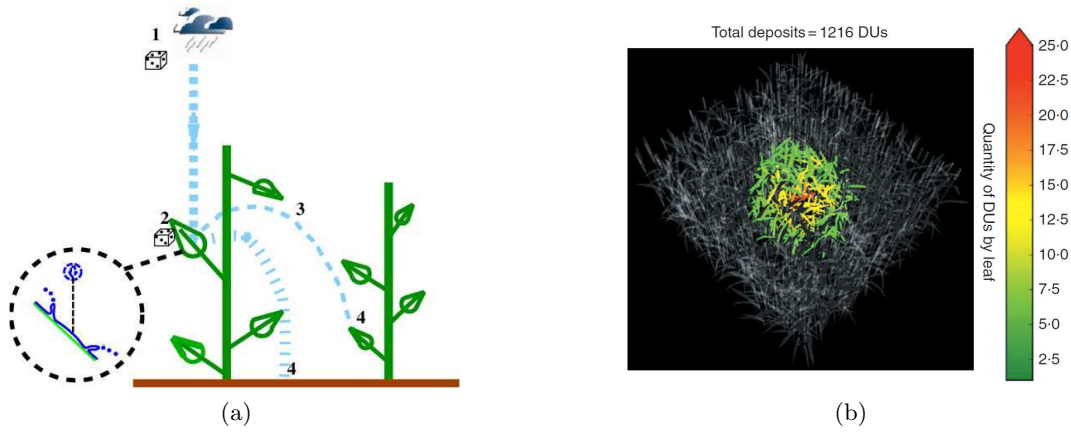
Figure 1.4: (a) Schematic representation of the interaction between raindrops and canopy elements. One iteration step of a Monte-Carlo integration modelling water transfer by rain-splash is shown: (1) sampling of the raindrops (2) the interception of the raindrop by an element of the canopy structure, followed by the production of the splash droplets and sampling of their characteristics (3) calculation of the curvilinear trajectories of the droplets (4) interception of each droplet by either the elements of the canopy or the ground. The model simulates stages (1), (2), (3) and (4). [Adapted from Saint-Jean et al. (2004) ]. (b) Simulation of foliar fungal epidemics using functional-structural plant models. Distribution of dispersal units (DU) after one dispersal event due to rain, with source leaf indicated in pink on the figure, on a wheat cultivar. [Adapted from Garin et al. (2014) ].
