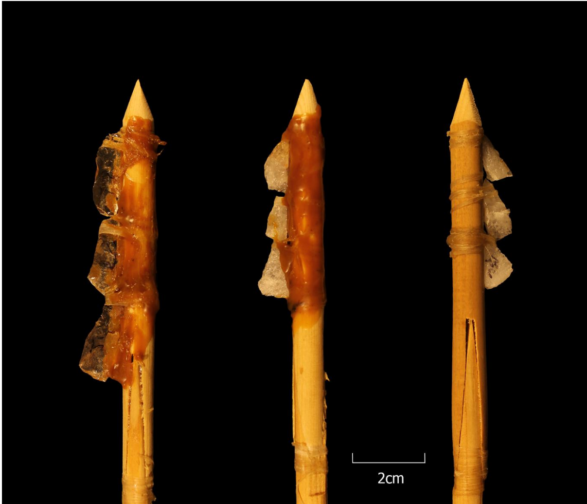
13 Fig. 3 Examples of barbed arrows before the experiment. Left: sinew and adhesive (Exp. 86/45), middle: 14 adhesive (spruce resin and beeswax) only (86/51), right: sinew only (86/53)
