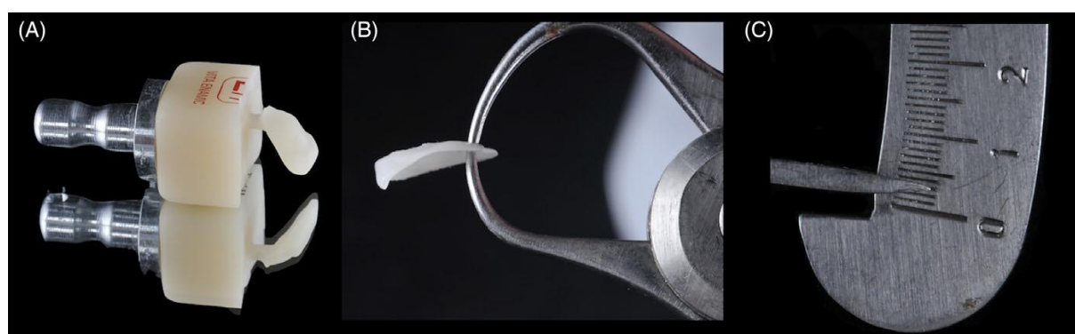
Fig. 9. A-C: A 0.2 mm-thick PICN posterior occlusal table top just after milling (Vita Enamic). Pictures were reprinted by permission of SAGE Publications Inc from Mainjot et al. 13
